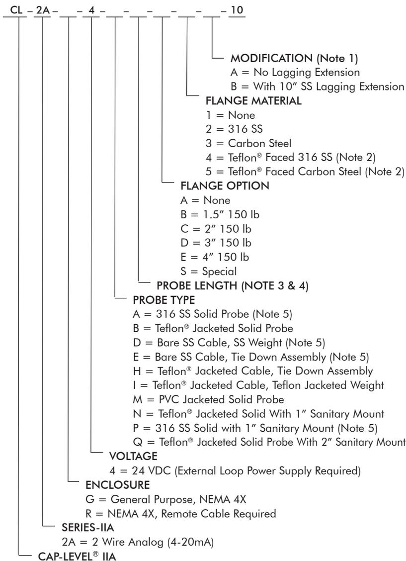
Note 1. Lagging assembly is used for high temperature applications.
