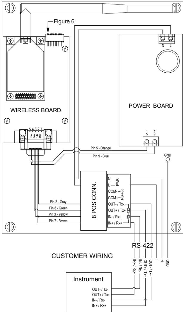
Figure 3: Wiring Diagram RS-485 (MODBUS)
