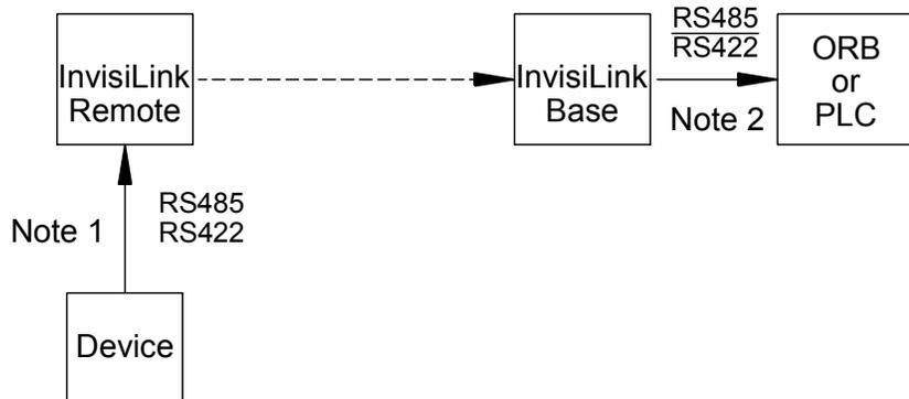
Figure 7. Point-to-Point (Multi Device)
