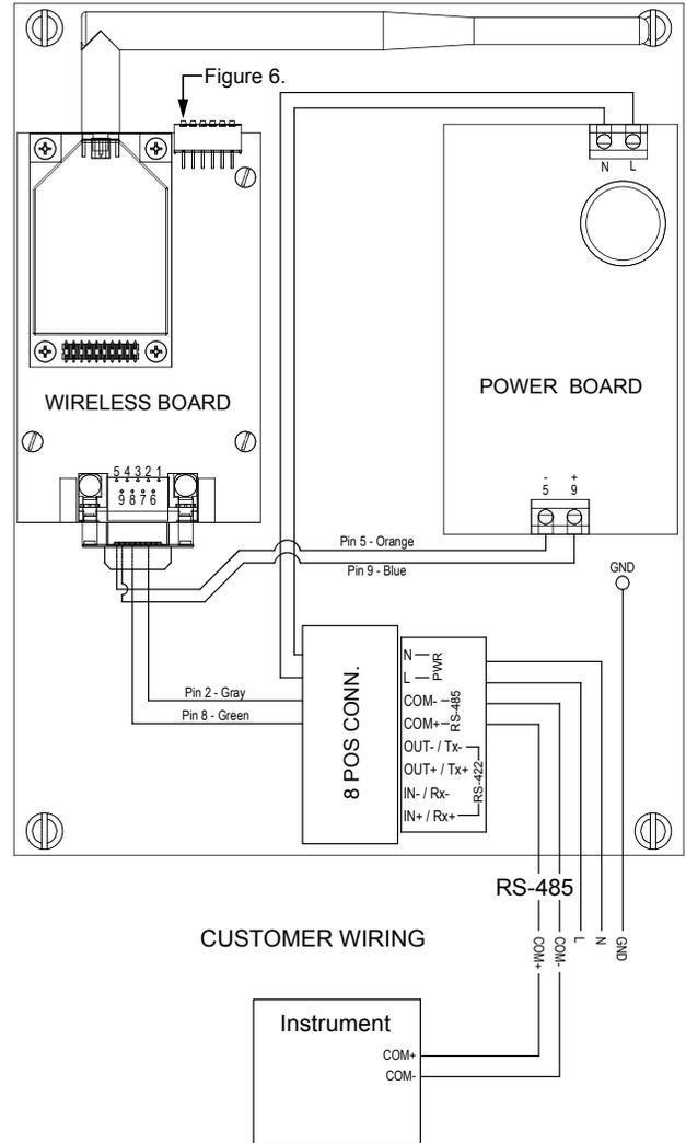
Figure 4: Wiring Diagram RS-422 with 4-20 mA Input Box
